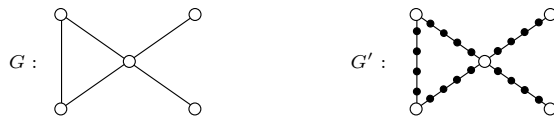
Fig. 1: An example of the transformation of a CLIQUE instance with k = 3 into a BICONNECTED SUBGRAPH instance with k' = 15 . White vertices in G' belong to V_1 , black vertices to V_2 .
