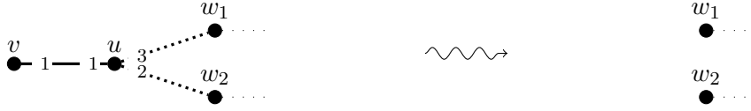
Figure 4.4: An example showing Reduction Rule 4.5 . Node v has u as its only neighbor. Node v is the single first preference of u . As Reduction Rule 4.4 is not applicable the dotted edges were already deleted and cannot exist. Hence, the edge \{u, v\} must be in the matching and nodes u and v can be deleted.
