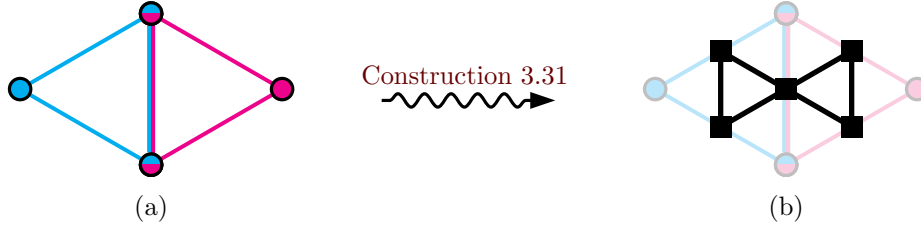
Figure 3.7: Illustration to Construction 3.31 . (a) Example graph G of the input instance \mathcal{I} = (G, c, \mathcal{H}, k) . The subgraphs induced by the habitats in \mathcal{H} are marked by differing colors. (b) Depicted in black, the graph G' obtained from G using Construction 3.31 . For illustration, the graph G of the input instance is faintly visible in the background.
